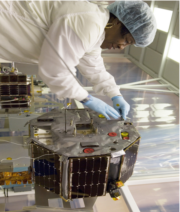
Helen Johnson, a spacecraft technician at NASA's Goddard Space Flight Center, works on one of the three tiny Space Technology 5 spacecraft in preparation for its technology validation mission.
