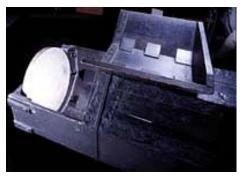
repolished often. The base of the telescope could be opened and the mirror easily removed. Another mirror was always on hand to use while the first was being polished.
